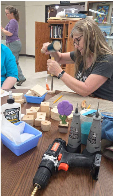
Left: Marlene adding stop-cuts with a gouge and mallet.
